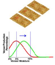
Shifting production to the left demonstrates the increased drying capacity as veneers shift from Overdry to an operator controlled Moisture Content (15%)
