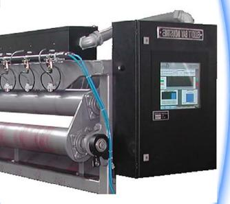
Advanced moisture level settings include parameters for perimeter moisture masking on the veneer edges, moisture pocket size, and average moisture levels
